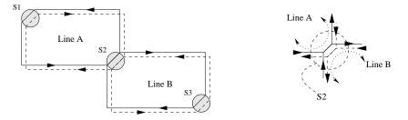
where Line A and Line B indicate the two underground lines (each one with two directions, clockwise and anti-clockwise), and S1, S2, and S3 are the three stations. Notice that in station S2 tracks are common, in both directions, for Line A and Line B (right-hand side picture).
